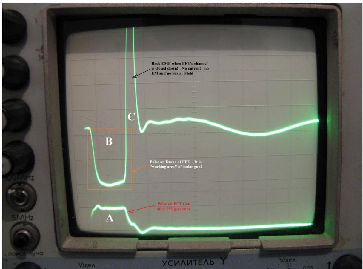
“A” is the pulse on the Gate (from 555 IC) of the power transistor and “B” is its drain response. In this area (in B) we have pulsed current where magnetic scalar field is generated. Note that “C” is just Back EMF and it is almost no current this time via cylindrical pipes – so no scalar field is generated in C area.
